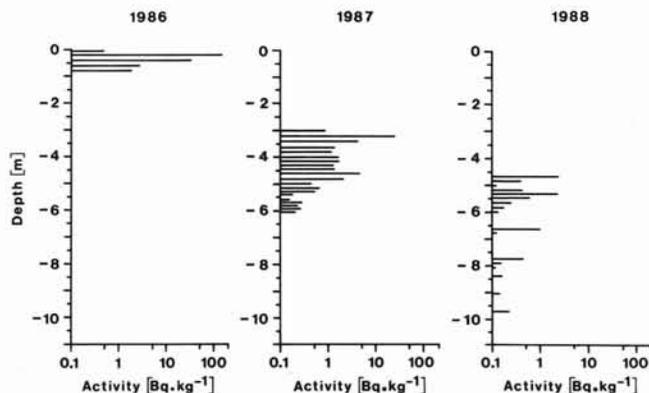
Fig. 1 - Gross-beta-activity of representative vertical snow profiles in the years 1986, 1987 and 1988 on Kesselwandferner (Ötztal Alps, Austria). Depth zero represents the surface at the respective times of sampling. Dates of sampling: July 1986, August 1987, July 1988, dates of measurement: August 1986, September-December 1987, September-December 1988.
