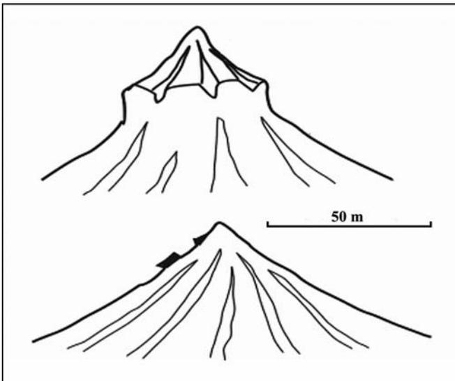
FIG. 4 - Morphological differences in the surfaces of the two piles of dross.
