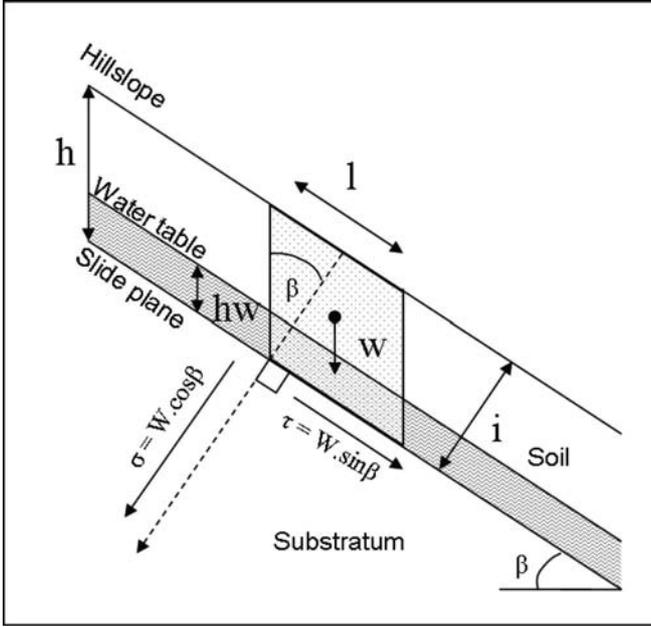
FIG. 2 - Infinite slope stability model, where the resisting force holding the block in place is given by  $W$  (mass \* the gravitational force) multiplied by the slope angle cosines. The driving force is  $W \sin \beta$  (inspired by Selby1993).
