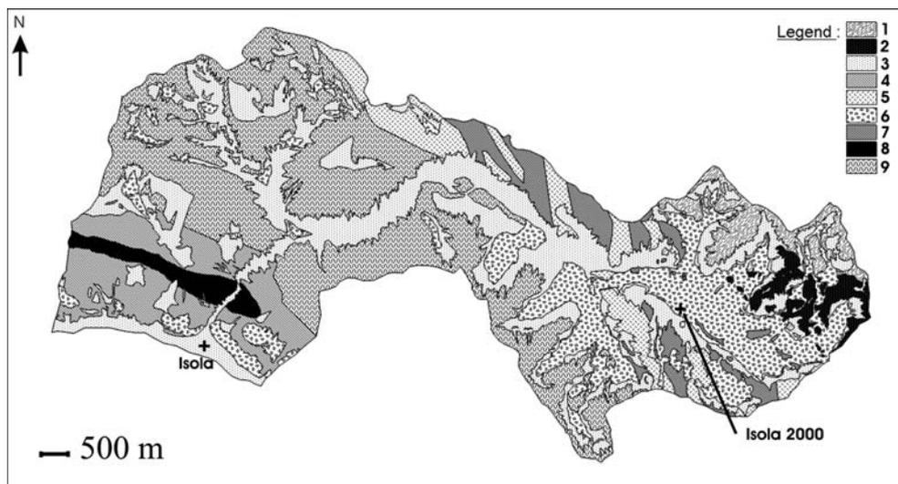
FIG. 5 - Geological map of the Isola catchment area. Occidental Unit: (1) Gneiss and migmatites (Anelle formation), (2) Diorite quartzite, (3) Gneiss and migmatite (Rabuons formation); Oriental Unit: (4) Embrechite, (5) Gneiss (Malivern Chastillon formation), (6) Anatexite, (7) Granite; Recent formation: (8) Glaciofluvial deposit, (9) Alluviums. UTM32 projection.
