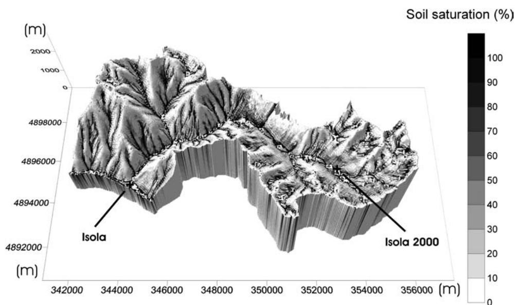
FIG. 6 - Soil saturation on the Isola catchment, (Maritim Alps, France) for a 20-year return rainfall event, approximately 60 min after the beginning of the rainfall. UTM32 projection.
