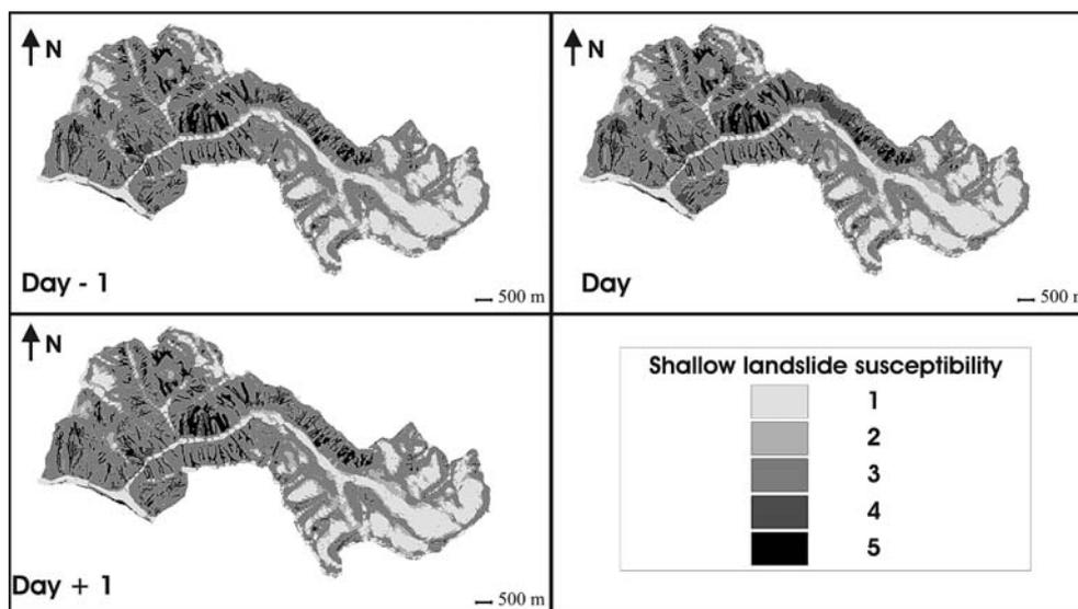
FIG. 1 - Isola catchment area susceptibility map for the shallow landslide (Risser & alii, 2007). Shallow landslide susceptibility legend: (1) low (FS > 1.8), (2) Low-Moderate (1.8 > FS > 1.3), (3) Moderate (1.8 > FS > 1.3 and talweg zone), (4) Moderate-High (FS < 1), (5) High (FS < 1 and talweg zone).
