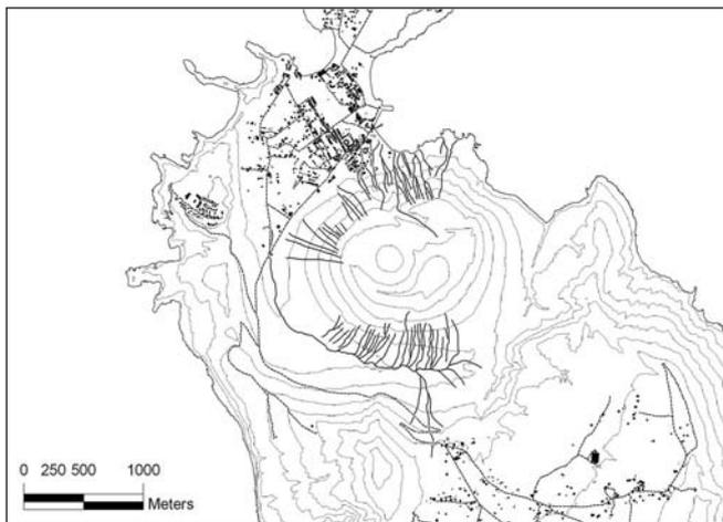
FIG. 3 - Stream/gully network (grey lines) as mapped in 1958 (IGM 1:25,000 map) with the superimposition of the urbanized area of Vulcano Porto as reported in the 1990 CTR (dashed dark grey lines are paved roads, black polygons are buildings); contour interval for elevation lines (pale grey) is 50 m.
