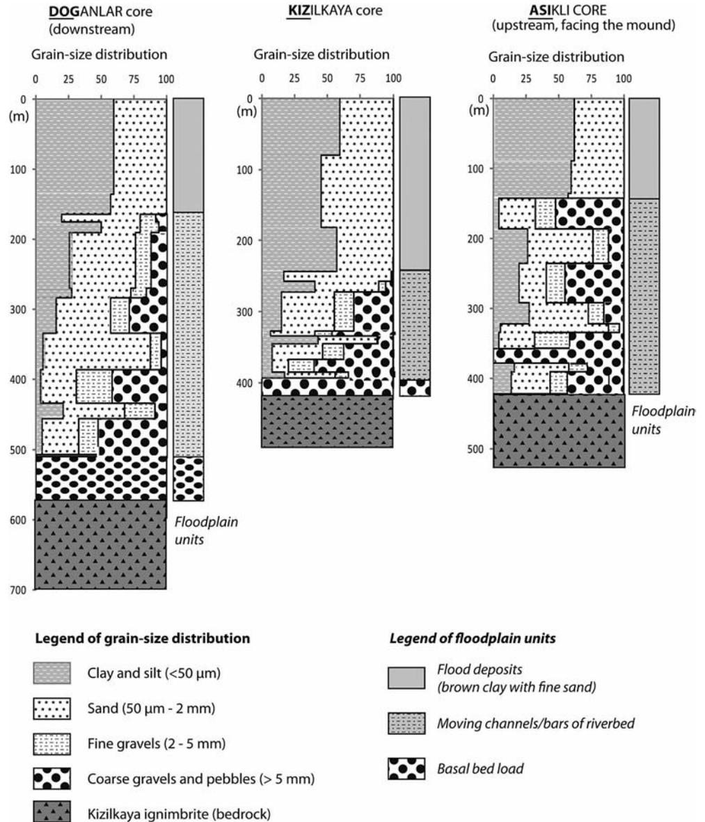
Aşıklı mound downstream to the Doğanlar village facing Kızilkaya village. The 64 mm diameter cores were extracted using a rotary and hydraulic Craelius XC-SH truck mounted drill. Cores were sub-sampled at the coring spots, with intervals based on the facies and estimated grain size of the stratigraphic units identified during the coring process. Samples were sent to Laboratoire de Géographie Physique (LGP) in Meudon (France) for analyses.
