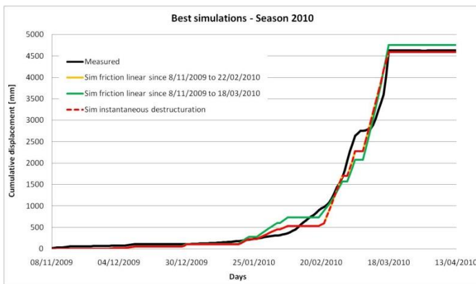
Figure 5: Comparison between cumulative snow glide measured and the three best simulations of Season 2010: simulation with friction angle varying linearly from the first to the last day, simulation with friction angle varying linearly from the first day 22 February 2010, simulation with instantaneous destructuration on 22 February 2010.
